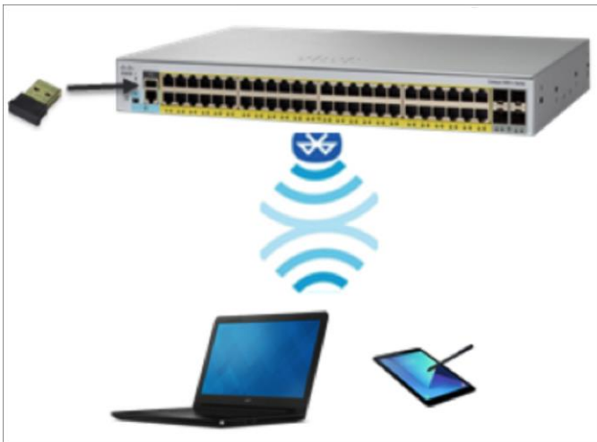
Figure 2. Over-the-air switch access using Bluetooth
